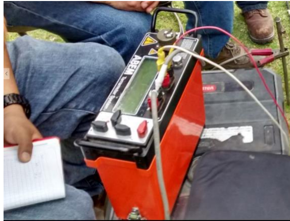
Fig 4: Picture showing Terrameter and other field gadgets
