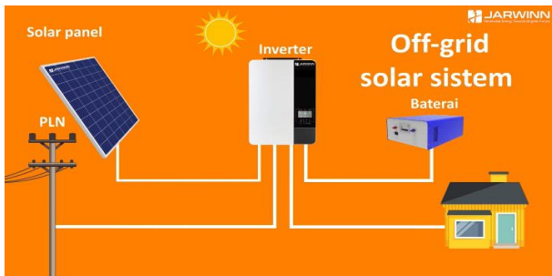
Gambar 7. PLTS Off Grid [14]
