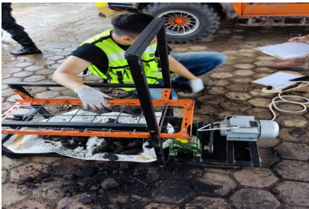
Gambar 9. Pengujian Model Vibrating Screen
