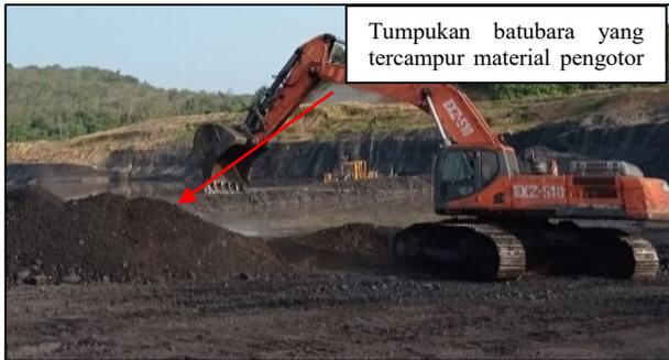
**Gambar 2.** Proses *coal cleaning*
