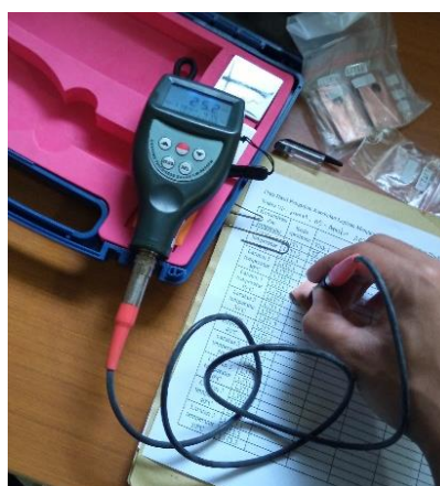
Figure 3. Coating Thickness Test
