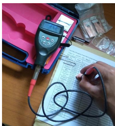
Figure 3. Coating Thickness Test
