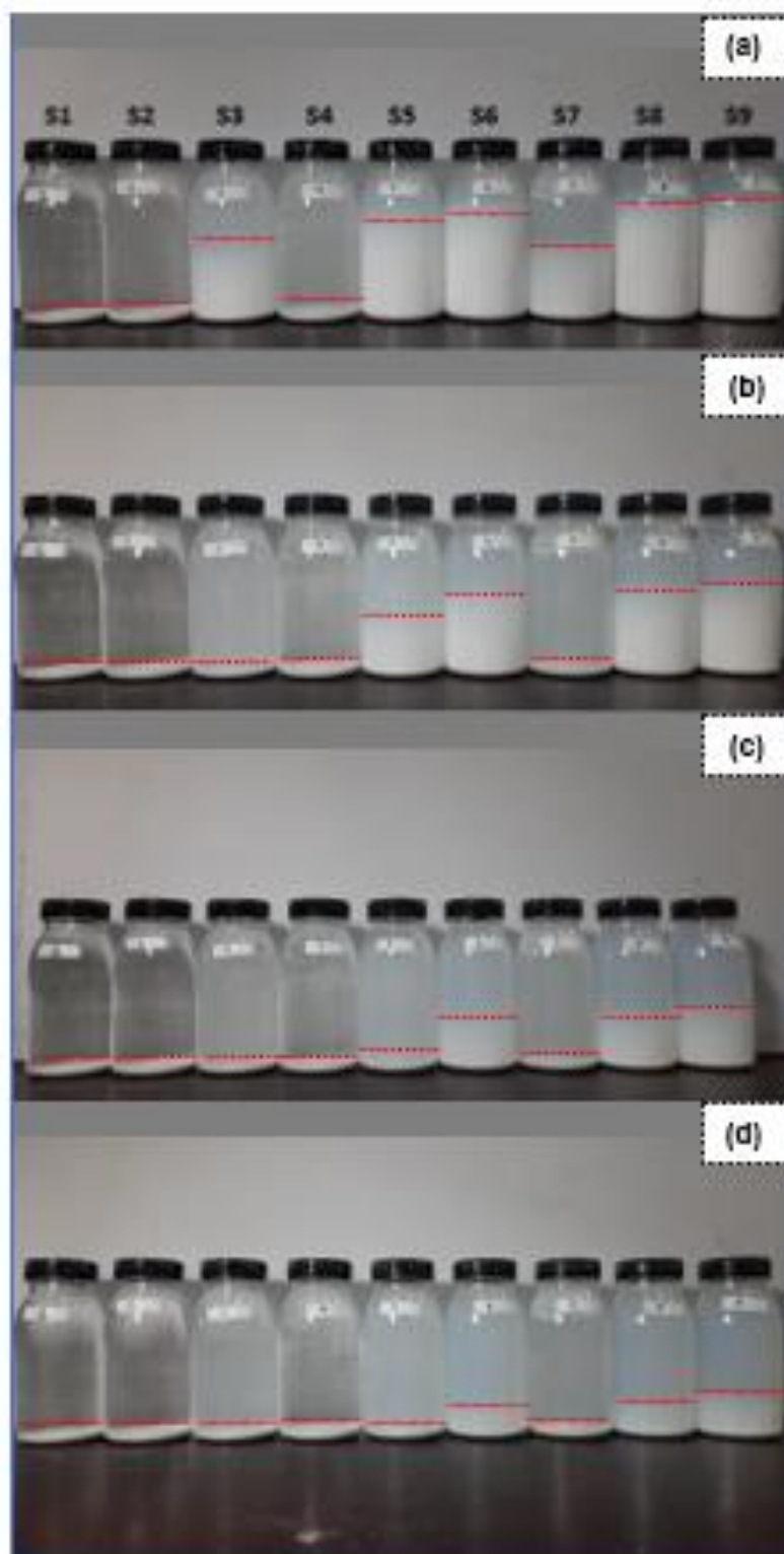
Figure 5. The photographs of Al_2O_3-TiO_2 /Water hybrid nanofluids stability; (a) One week, (b). Two weeks, (c). Three weeks, and (d). Four weeks after preparation
