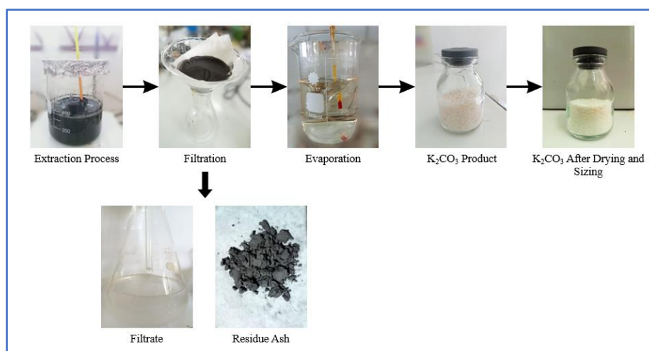
Figure 2. K_2CO_3 Extraction from empty oil palm bunch ash (EPFB)
