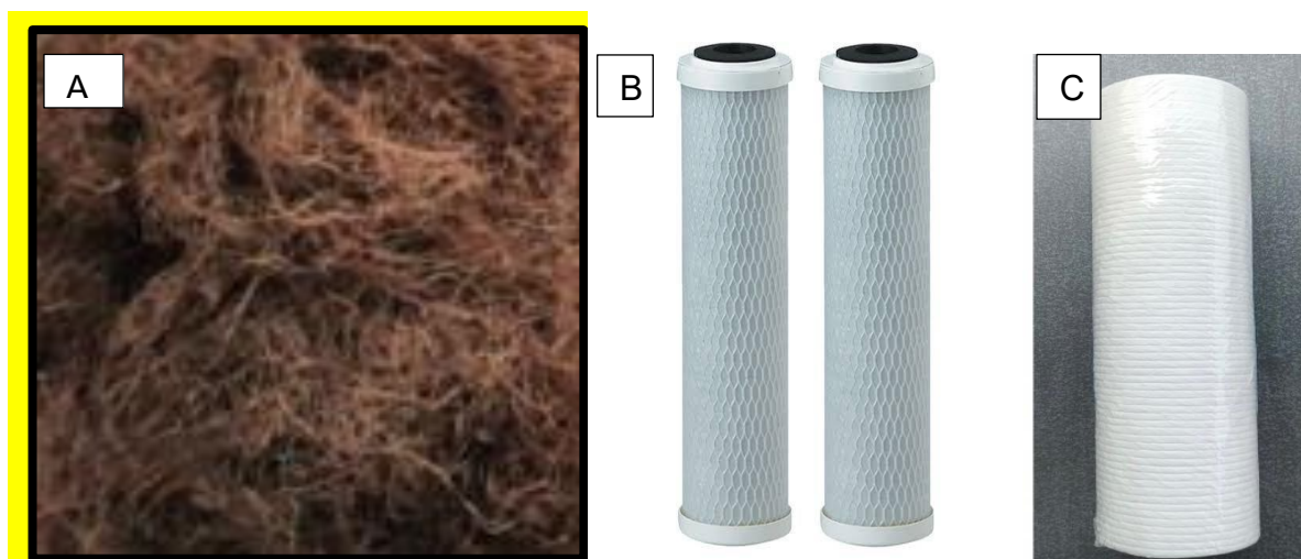
Figure 1. Adsorbents and polypropylene sediment filter. A. Oil palm fiber. B. Activated carbon block. C. Polypropylene sediment filter.
