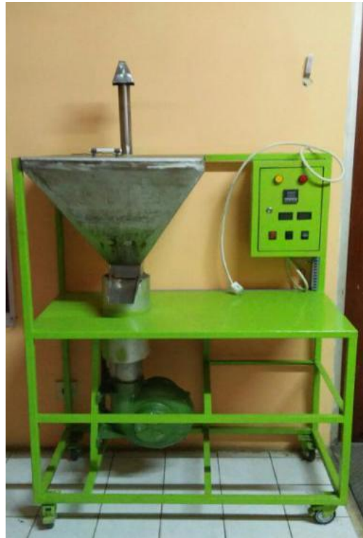
Gambar 1. Alat Sangrai Kopi Tipe Fluidisasi ( Fluidized Coffee Roaster )
