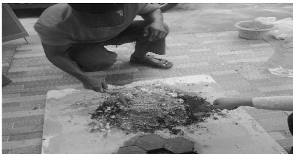
Gambar 5. Kegiatan Pencampuran Bahan Baku *Paving block* Campuran Sampah Plastik
