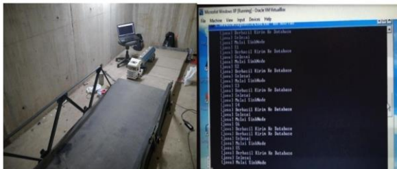
Gambar 7 Purwarupa SHMS Single Degree of Freedom (Wibawa, dkk., 2020)
