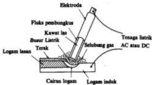
Gambar 1 Shield metal arc welding [1].
