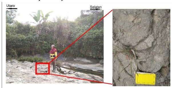
Gambar 5. LP.. Batugamping Wackestone
