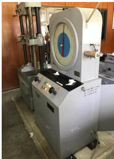
Gambar 3 Mesin Uji Tarik : Hydraulic Universal Material Tester
