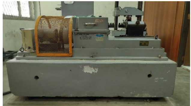
Gambar 4 Mesin Uji Fatik : Torsion Repeated and Bending Fatigue Machine.
