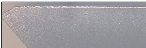
V_c = 156.25 \text{ m/min} (Keausan 0.0108 mm)
