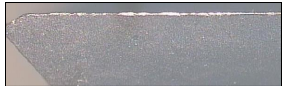
a_r = 0.51 \text{ mm} (Keausan 0.0158 mm)
