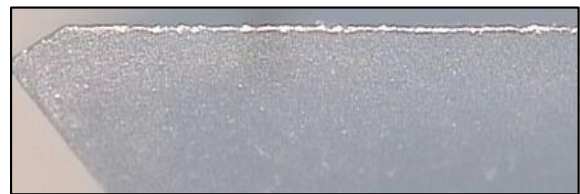
a_x = 3.54 \text{ mm} (Keausan 0.0126 mm)
