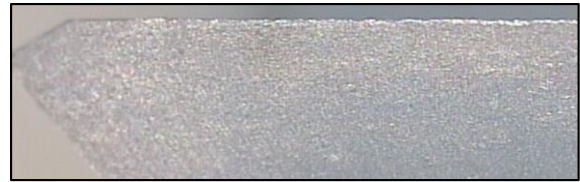
f_z = 0.025 \text{ mm/flute} (Keausan 0.0102 mm)
