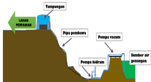
Gambar 2 Prinsip kerja Pompa vacydrum
