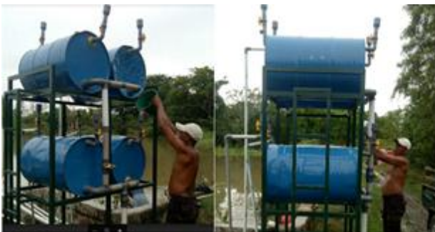
Gambar 9 Pengujian Pompa Vachydram
