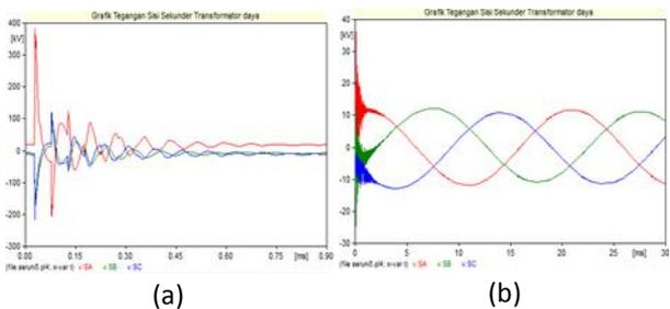
Figure 7. Voltage magnitude at transformer secondary side, lightning strike to AS node (a) arrester uninstalled, and (b) arrester installed
