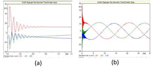
Figure 9. Voltage magnitude at transformer secondary side, lighting strike to CS node (a) arrester uninstalled, and (b) arrester installed
