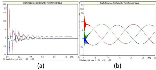
Figure 4. Voltage magnitude at transformer secondary side, lightning strike to AM node (a) arrester uninstalled, and (b) arrester installed
