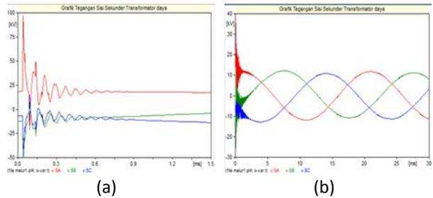
Figure 5. Voltage magnitude at transformer secondary side, lightning strike to BM node (a) arrester uninstalled, and (b) arrester installed
