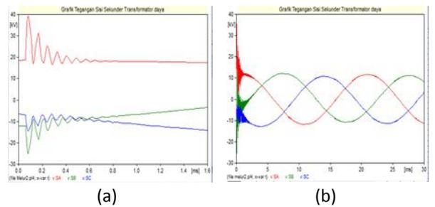
Figure 6. Voltage magnitude at transformer secondary side, lightning strike to CM node (a) arrester uninstalled, and (b) arrester installed
