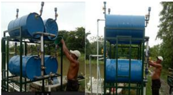
Gambar 9 Pengujian Pompa Vachydram
