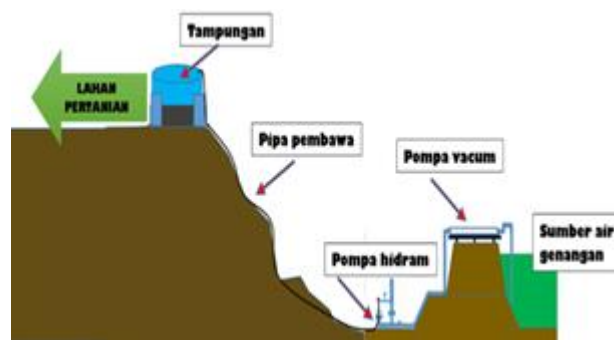
Gambar 2 Prinsip kerja Pompa vacydrum
