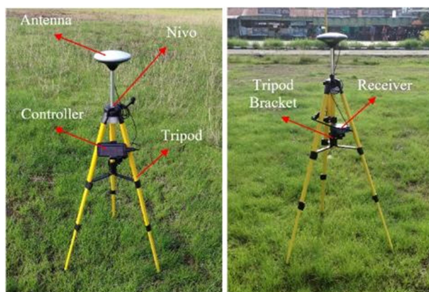
Gambar 7. Low-cost GNSS RTK hasil rancangan
